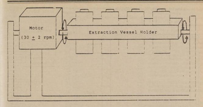
Figure 2: Rotary Agitation
