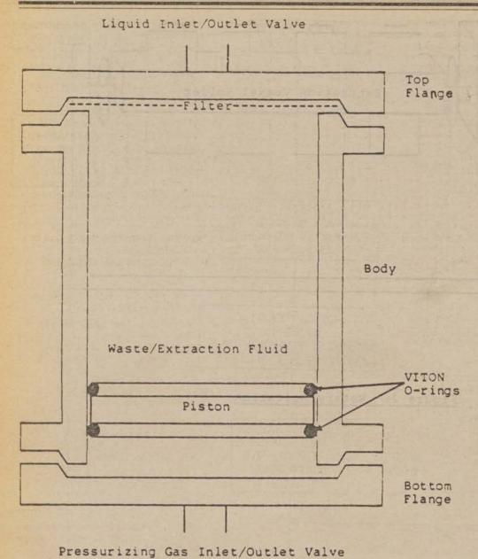
Figure 3: Zero-Headspace Extraction Vessel
