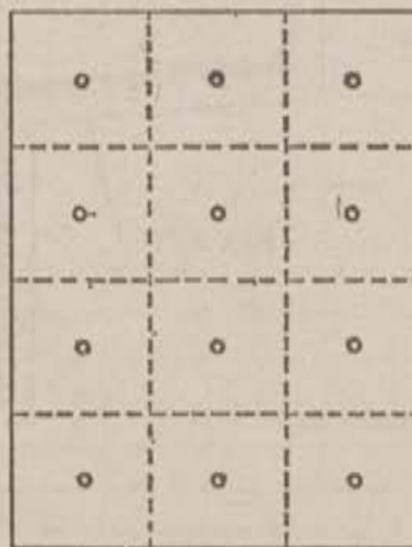
Figure 1-3. Cross section of rectangular stack divided into 12 equal areas, with traverse points at centroid of each area.
