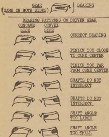
TOOTH BEARING OF SPIRAL BEVEL GEARS
